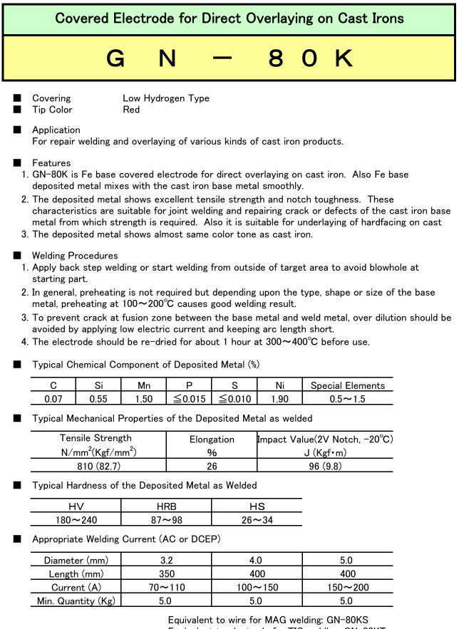
Equivalent to electrode for TIG welding: GN-80KT
